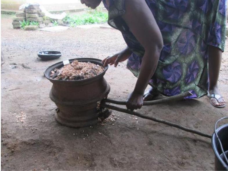
Figure 2: placing two small firewood sticks into the side hole
