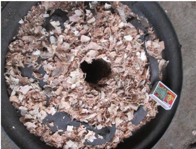
Figure 1: after sawdust is compacted and bottle is removed from the middle
