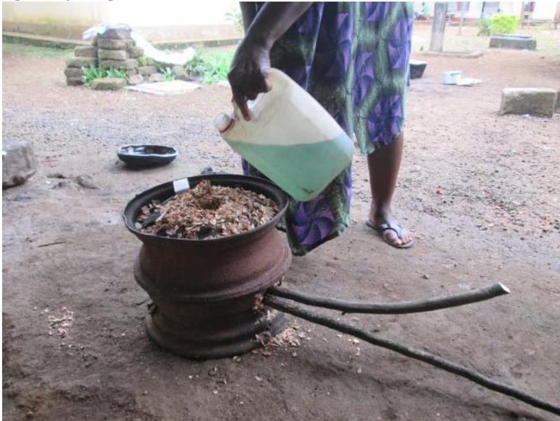
Figure 3: pouring kerosene into the top hole before lighting the stove with matches
