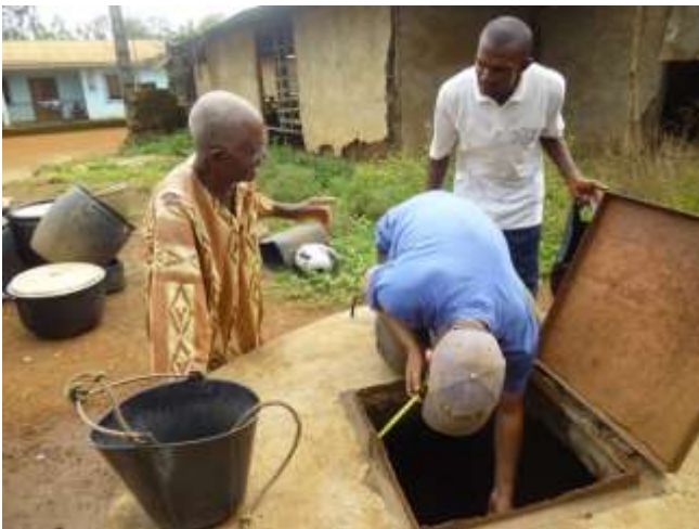
technique. Figure 21. Rogerio and Takor measuring depth of water in well during rainy season.
