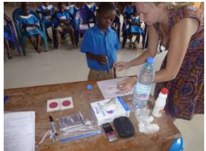
A participant uses 3M Petrifilm to test Besongabang well water for coliform and e-Coli.
